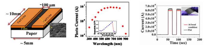
3.(a)Schematic of the wearable electronics based flexible photo detector, b) Spectral Response of the photo current (illumination intensity 120  $\mu$ W/cm2) Inset :Spectral dependence of the Responsivity. (C) Comparison of response of flexible photo detector in flat/bend condition
