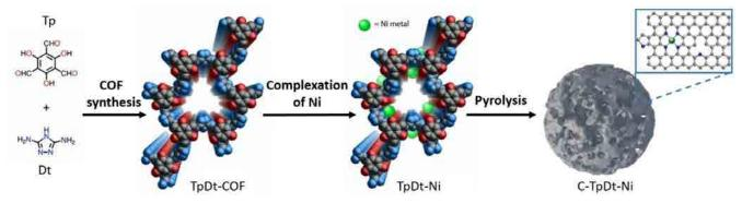
Figure 2. Scheme for the synthesis of C-TpDt-N (Ni-N-C catalysts).
