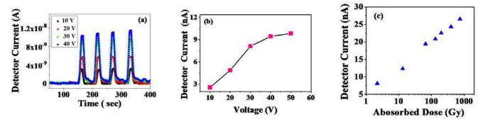
Figure 2: a) Current Response by γ ray detector (using Co-60 source) b) Voltage dependent current response by the detector c) Detector Current as function of absorbed dose
