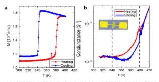
Figure 2: (a) M-T curve for the bare SCO nanoparticle showing a thermal hysteresis. (b) Conductance measurement of bare nanoparticle showing similar thermal hysteresis.
