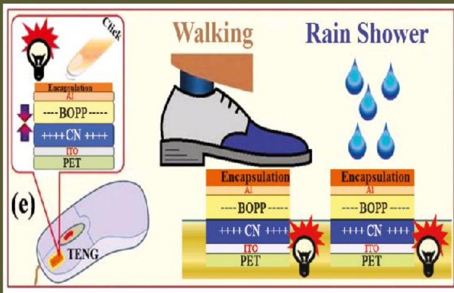
Schematic of 2D g-C 3 N 4 TENG based mechanical energy harvesting using human activities and rain shower etc.
