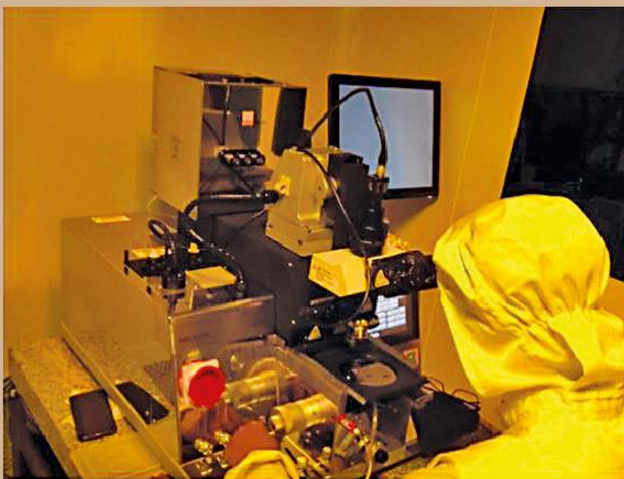
Student performing optical lithography in the Mask aligner.
