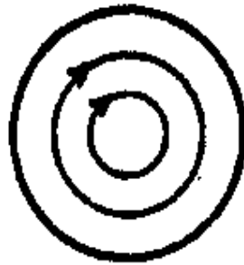
Figure 2.3: Types of simple domain arrangement in a small sphere with low anisotropy.
