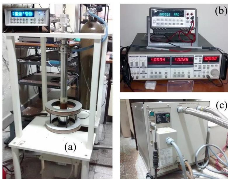
**Fig. 2.10:** (a) Cryostat; inset: Lakeshore 332 temperature controller. (b) SRS830 DSP lock in amplifier and Agilent 34401A digital multimeter. (c) Sumitomo SRDK-205 cryocooler.
