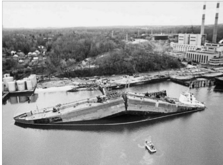
Figure 1.1: Around 90 out of 2700 ships manufactured by a U.S. Liberty Ship Building Program during World War II underwent serious fractures with some of them resulting in breaking completely into two halves. This picture is taken from the website [1].
