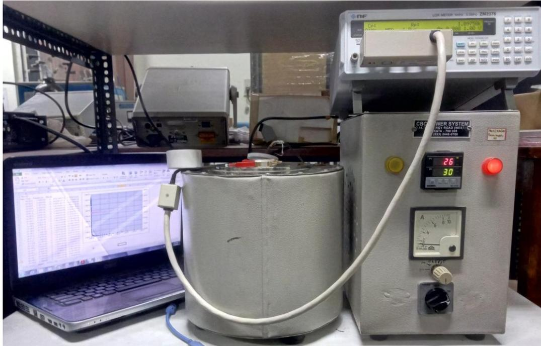
Fig. 2.17: Dielectric properties measurement setup.
