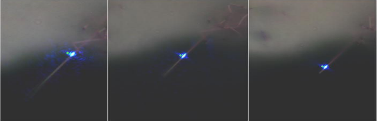
Figure 5. (b) A 488 nm Ar ion laser focused on a single cantilevered Ge NW at different positions.
