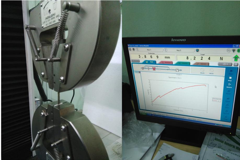
**Figure 2.12 INSTRON Model 3365 universal testing system**
