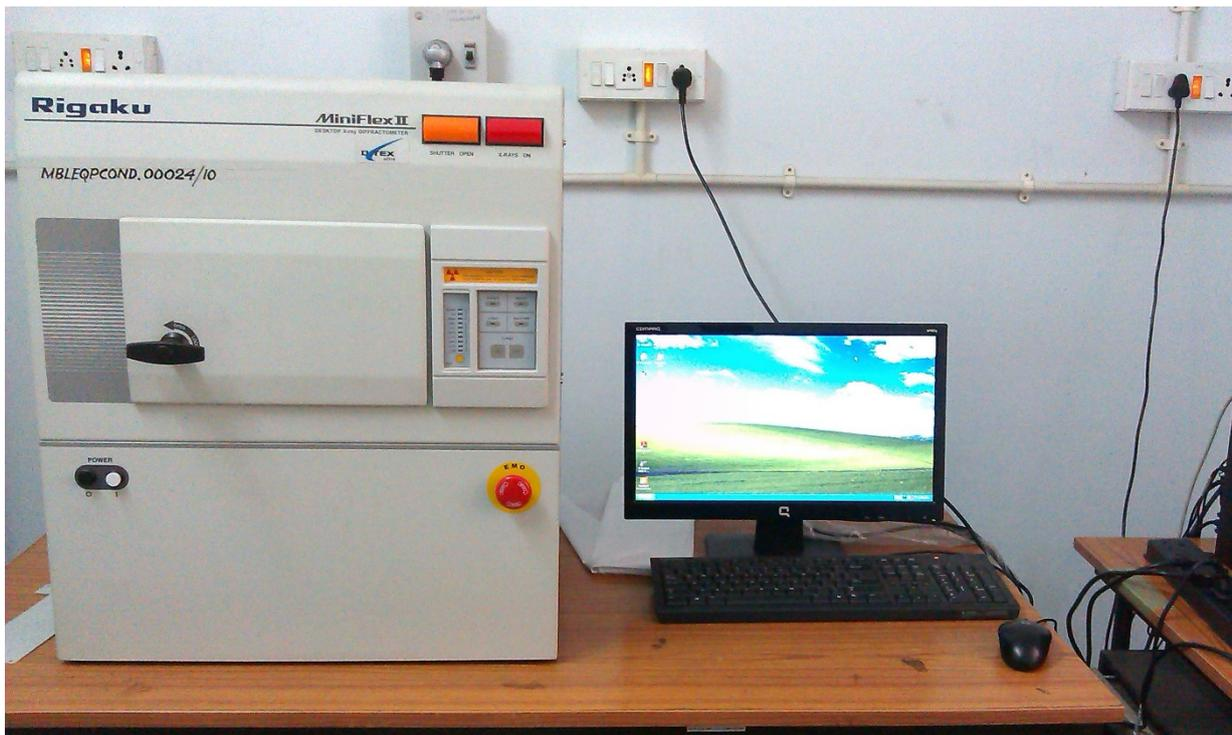
Figure 2.7 RIGAKU MiniFlex II diffractometer (XRD) unit [2.9]
