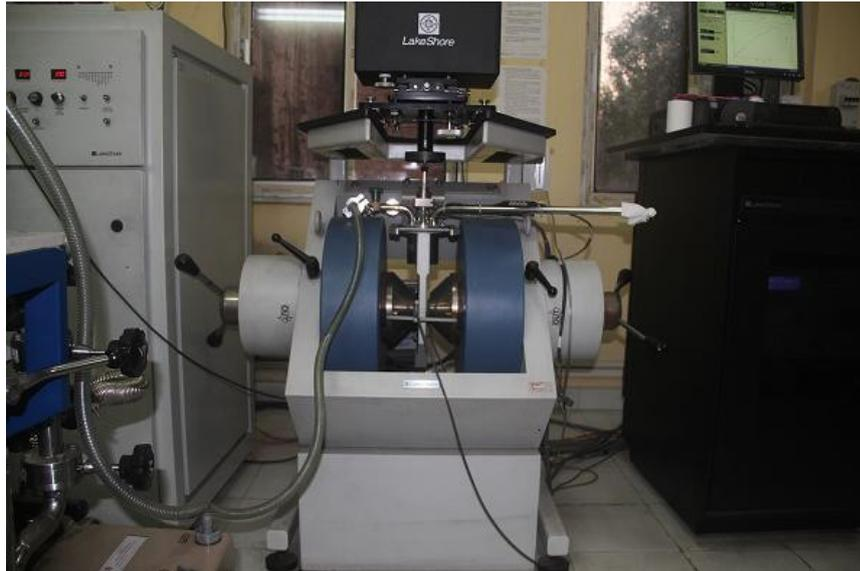
**Figure 2.11 Lake Shore Cryotronics 7400 VSM unit [2.21]**
