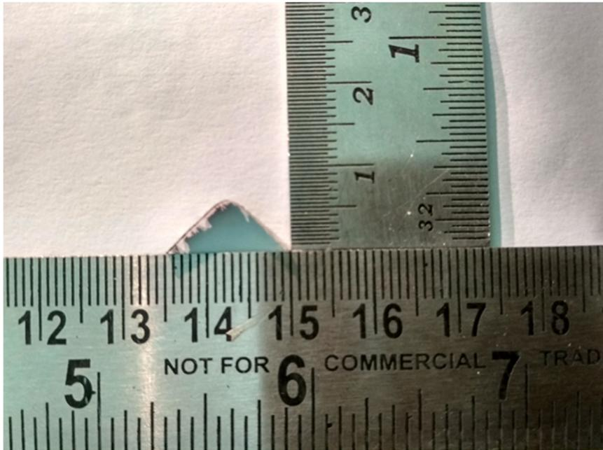
Figure 6.2 (a) Actuating part of FSMA microgripper system
