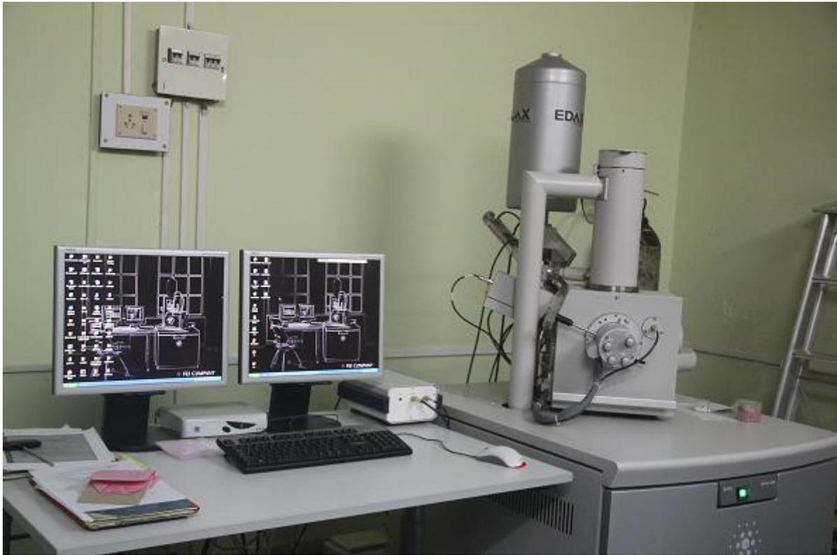
**Figure 2.5 Energy dispersive X-ray analysis (EDAX) instrument [2.5]**
