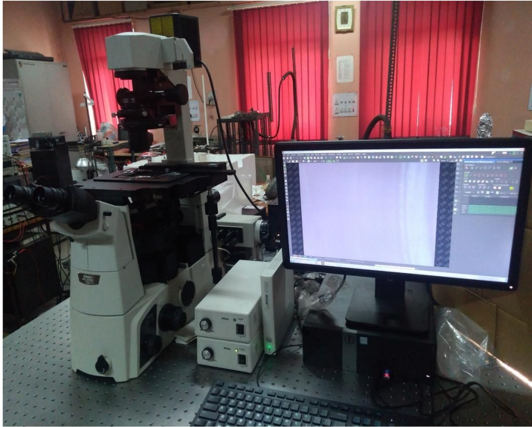
**Figure 2.14 Nikon Eclipse Ti-U inverted research microscope**
