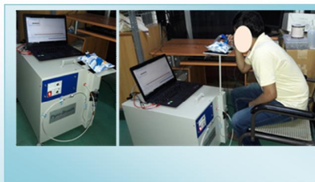
A prototype breath analyzer, so called “**Pyro-Breath**”, has been developed in the TRC project. The analyzer can diagnose stomach infection and ulcer disease by means of human breath analysis. Exhaled breath contains a large number of different molecular species with ultra-low concentrations in the levels of parts per billion (ppb) to parts per trillion (ppt). Some of these molecules and their isotopes are closely associated with the development of disease or metabolic disorder in human.
